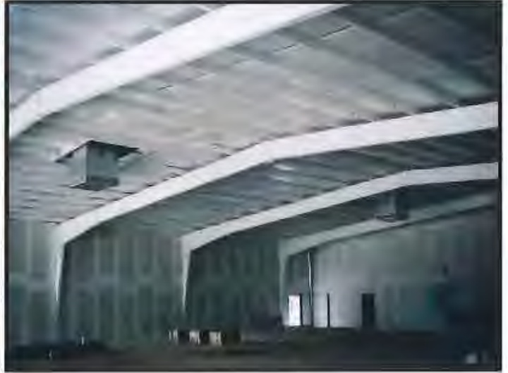
Numerous other Airplane Hangars—All Pre-Engineered Metal Buildings Sizes Ranged from 80'x80' up to 100'x150' and up to 28' Eave Heights
